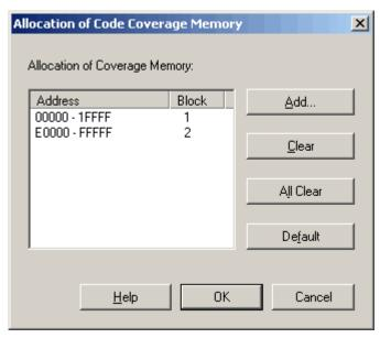
Figure 5.73 Allocation of Code Coverage Memory dialog box
